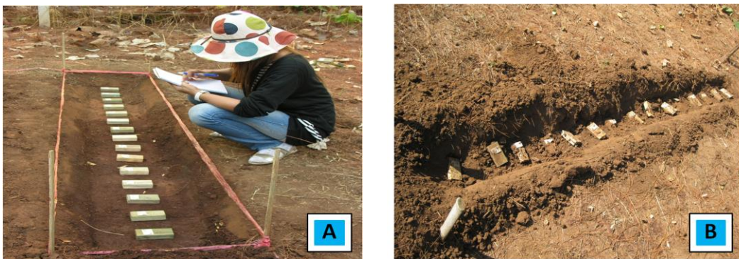
Figure 3. Under-ground durability testing of P. caribaea wood; (A) before and (B) after testing
