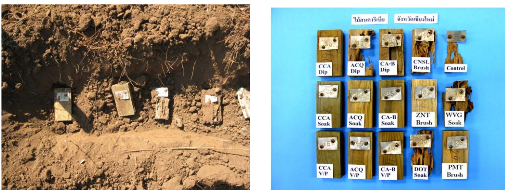
Figure 4. P. caribaea wood specimens after 10 months of exposure in under-ground durability testing
