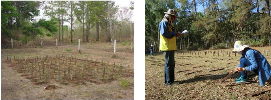
Figure 1. Natural durability testing and periodic inspection of treated P. caribaea wood
