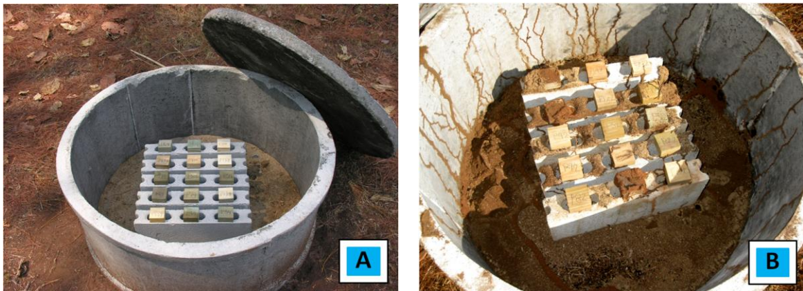
Figure 5. Field testing of durability of treated P. caribea wood in above-ground condition ; (A) before and (B) after testing
