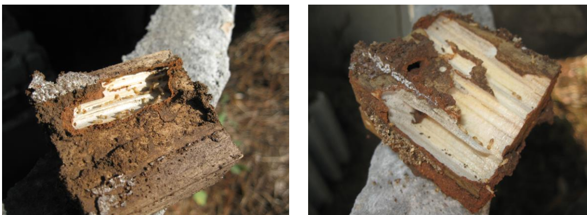
Figure 6. Pinus caribea wood specimens after 10 months of exposure
