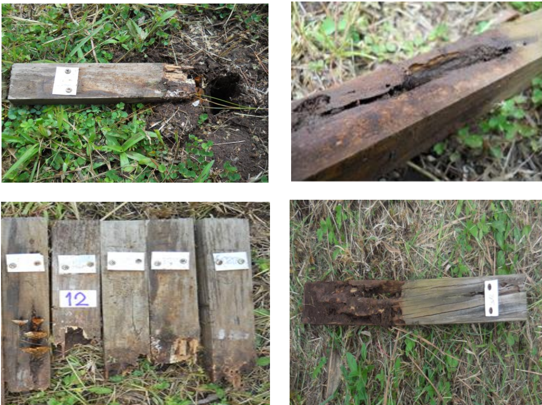
Figure 2. Failure of P. caribaea wood specimens in field testing for natural durability
